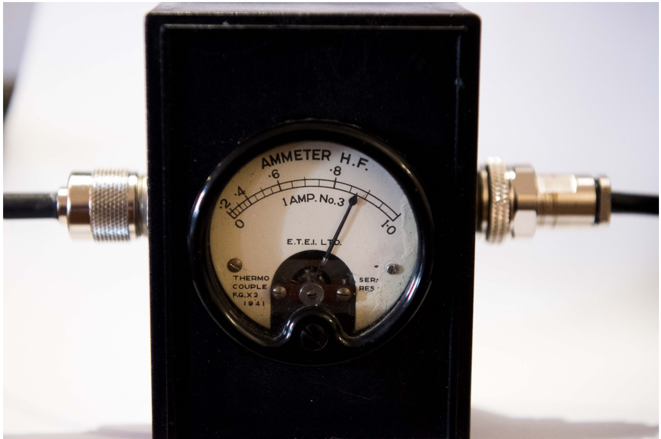
Pic. 26 The RF ammeter utilized in this test, a vintage thermocouple based instrument, able to measure RF currents, in the HF spectrum, up to 1A.
