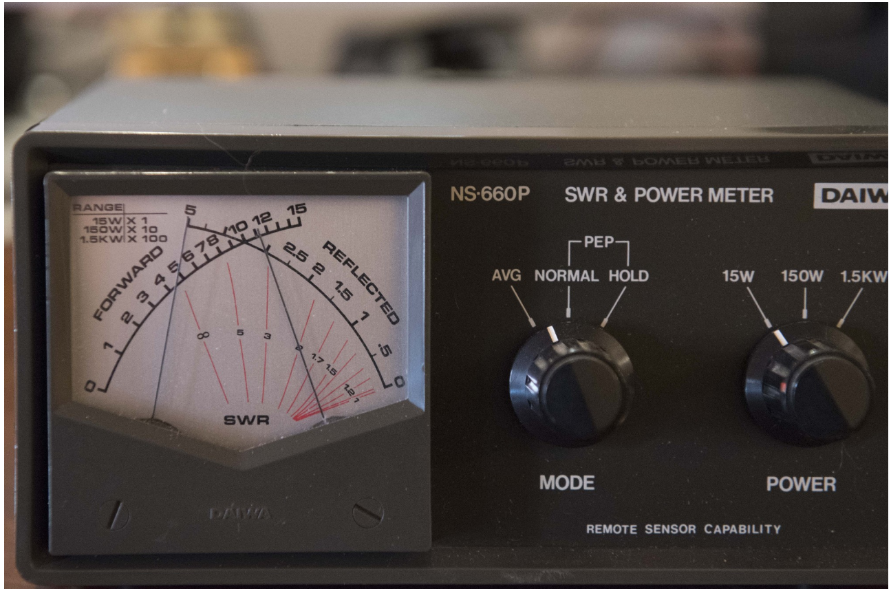
Pic. 20 Here the meter is just out of the tuner, on the ANT port side The forward power is slightly above 11W, while the reflected power is 5W.
