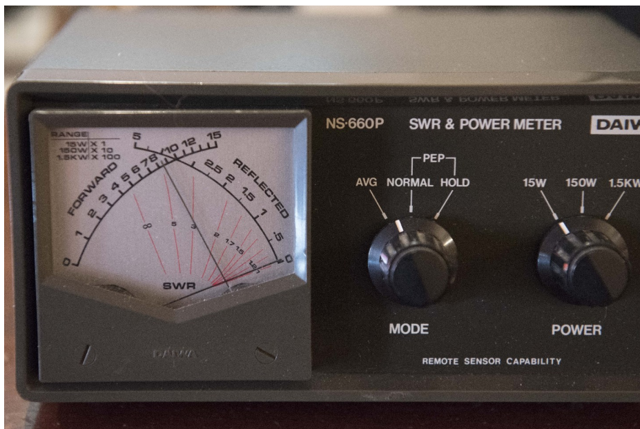
Pic. 19 The Daiwa NS-660P power meter used for this test here installed at the tuner input (RTX side). It shows 8,5W of forward power, with negligible reflected power.
